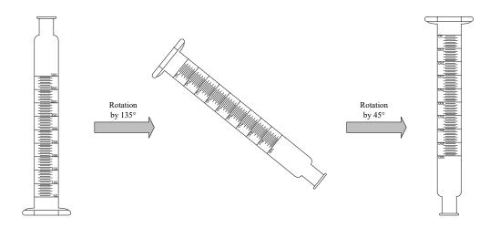
Figure 1: Pouring procedure.
