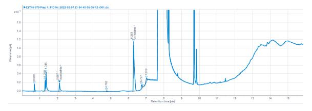
GC Chromatogram of Chlorantraniliprole 600 SC Formulation Sample containing 35.05 mg/mL (1752.6 mg/50mL) technical a.i. in DMAC
